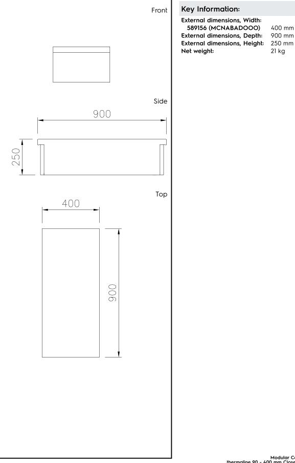
Modular Cooking Range Line thermaline 90 - 400 mm Closed Work top, 1 Side
